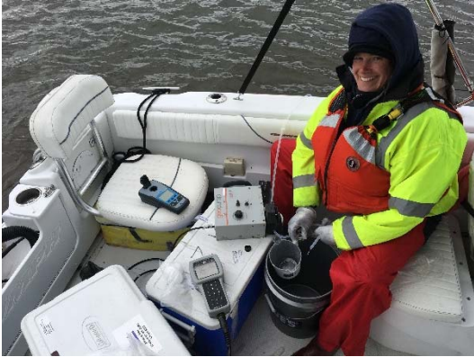
Surface water sampling with a peristaltic pump.
