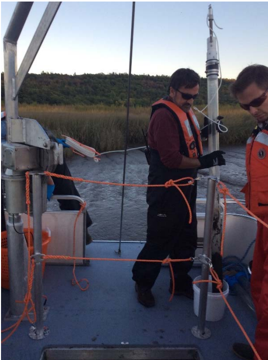
Push core method used to collect subtidal and intertidal sediment samples.
