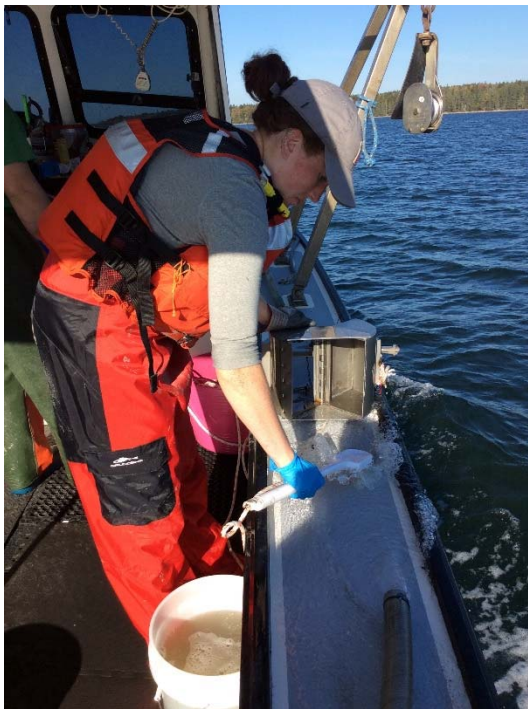
Decontaminating Ponar during subtidal sediment sampling.
