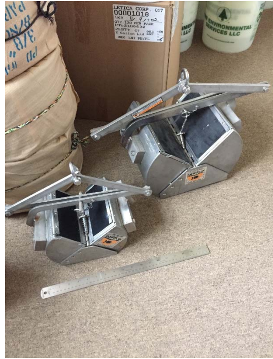
Two different sized Ponars used to collect subtidal sediment samples.
