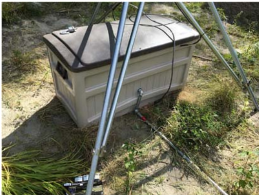
Turbidity meter equipment garden box
