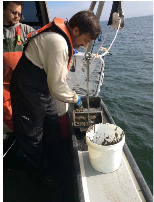
Ponar used to collect subtidal sediment samples.
