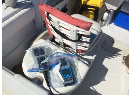
Water quality meter and turbidity meter used for taking surface water parameters.
