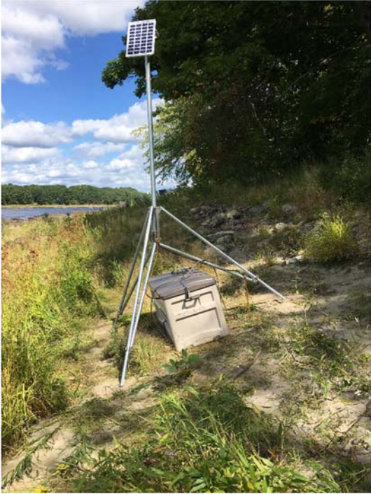
Turbidity meter equipment and solar power tripod installation
