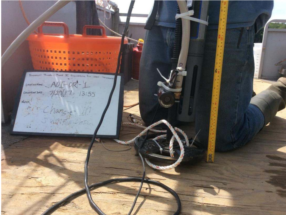
PHOTO 4: Adjusted and final phase 2 sampling method using weighted apparatus, sonde probe, single hose, and water camera for sample collection.
