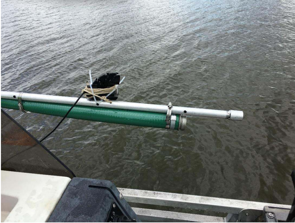
PHOTO 1: Phase 1 of sampling method using metal rods to extend sampling hose into water column.
