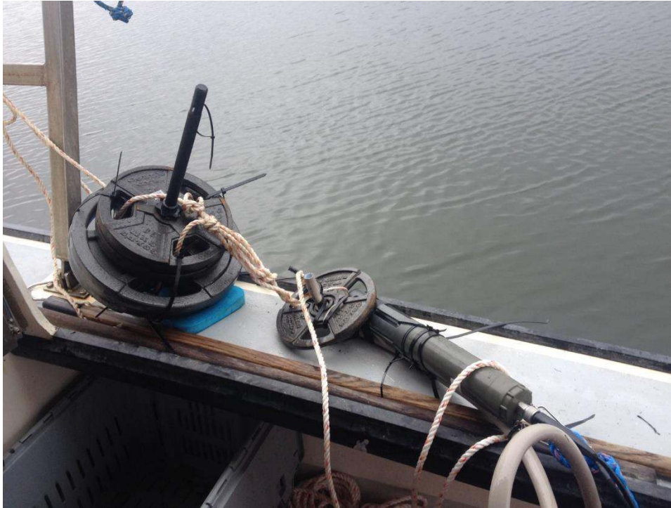
PHOTO 10: Sonde and hose apparatus used for the September 19, 2017 sampling event.
