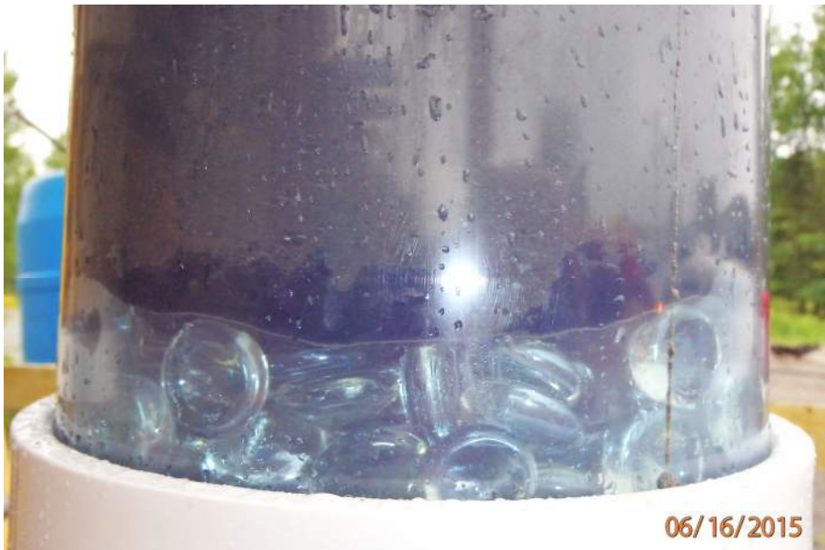
Photo 8: Sediment migration at filter fabric during dewatering.
