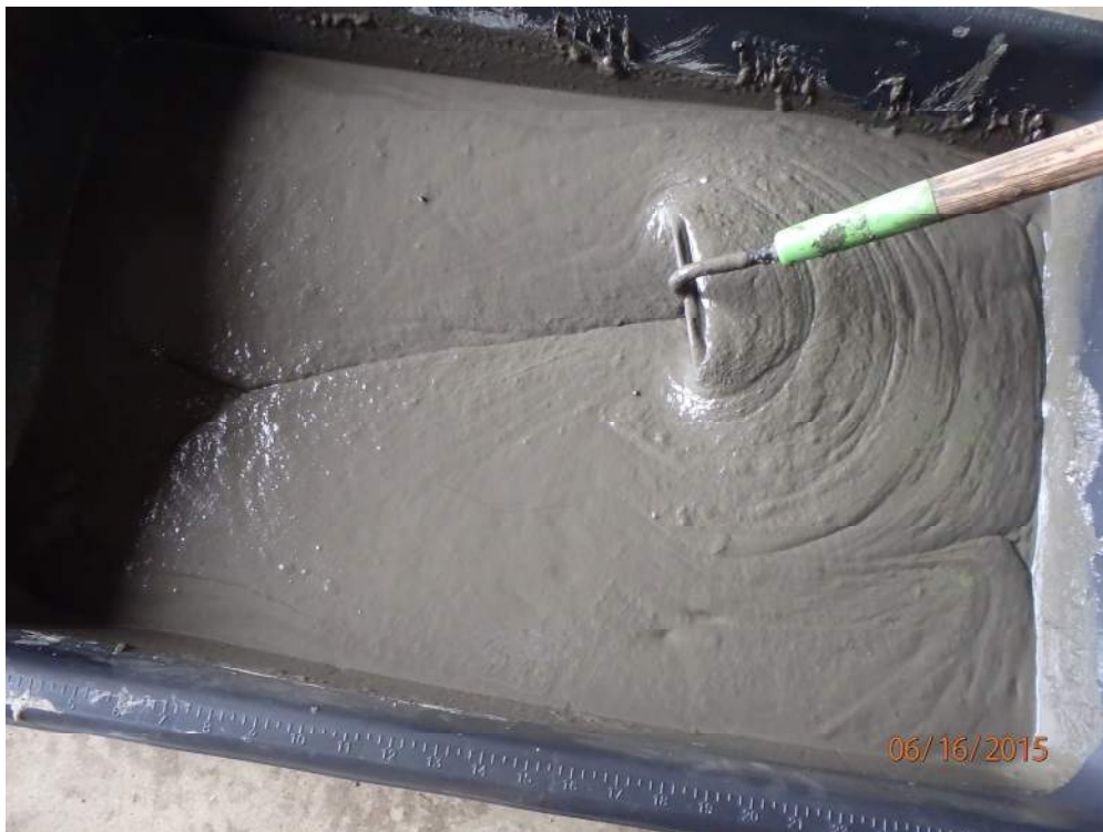
Photo 6: SD-SC-08, -09, -10 Composite, mixed to dredged consistency before dewatering.
