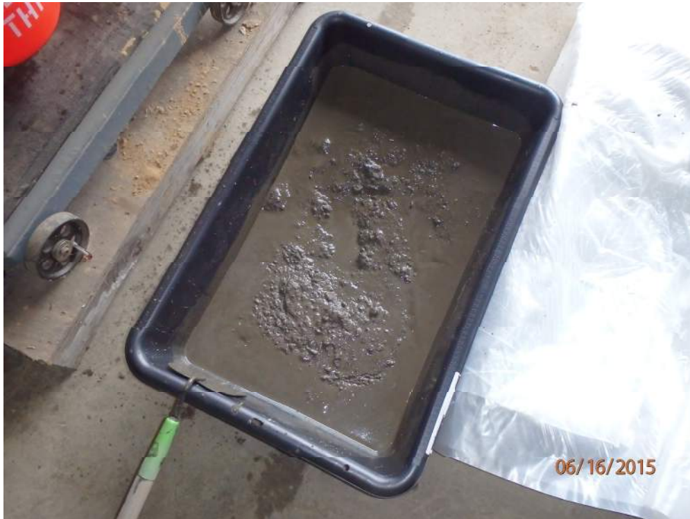
Photo 5: SD-SC-07, mixed to dredge consistency before dewatering.
