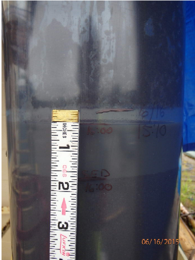
Photo 9: SD-SC-07, water and sediment levels in dewatering tube.
