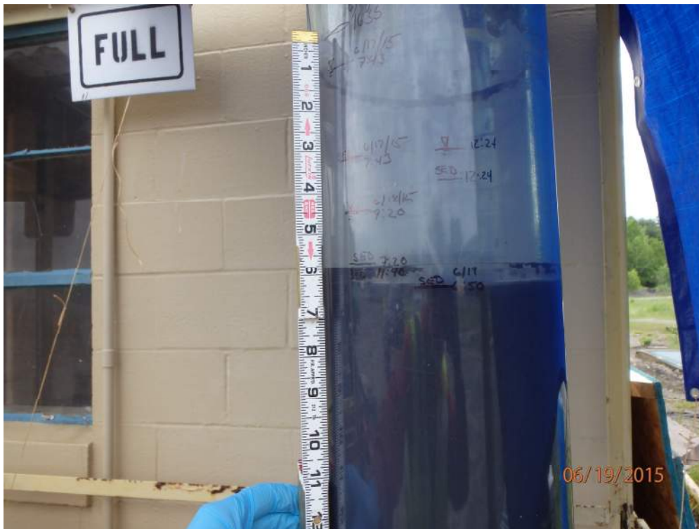
Photo 13: SD-SC-08, -09, -10 Composite dewatering test, approximately 62 hours test time.
