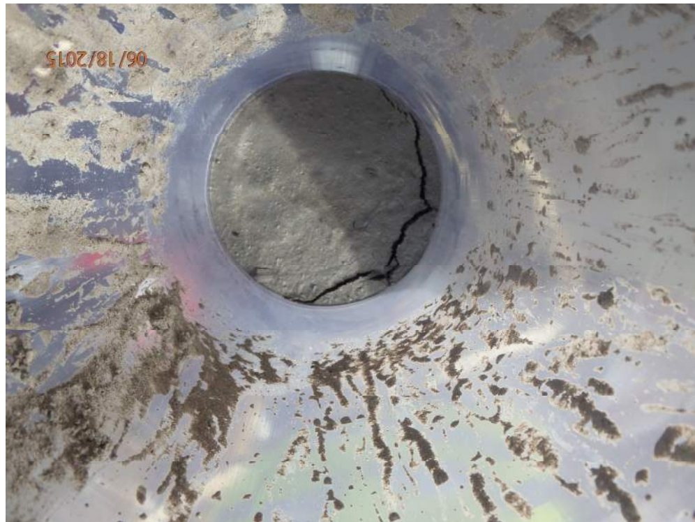
Photo 11: Top of SD-SC-07 dewatered sediment at completion of test.
