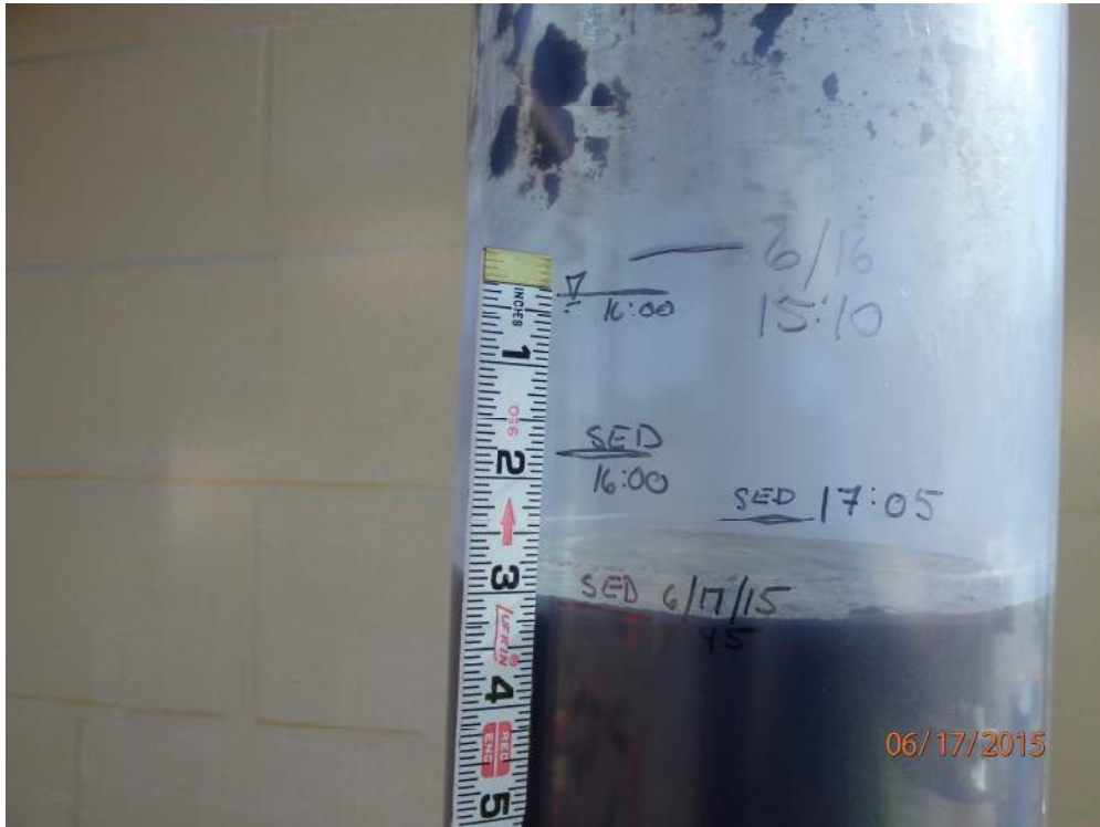
Photo 12: SD-SC-07 dewatering testing, additional measurements.
