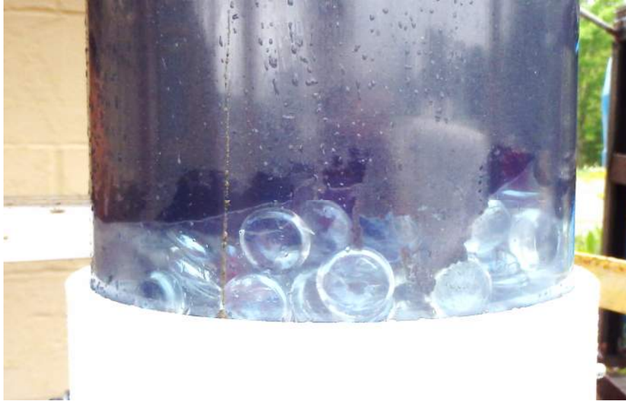
Photo 7: Sediment migration at filter fabric during dewatering.
