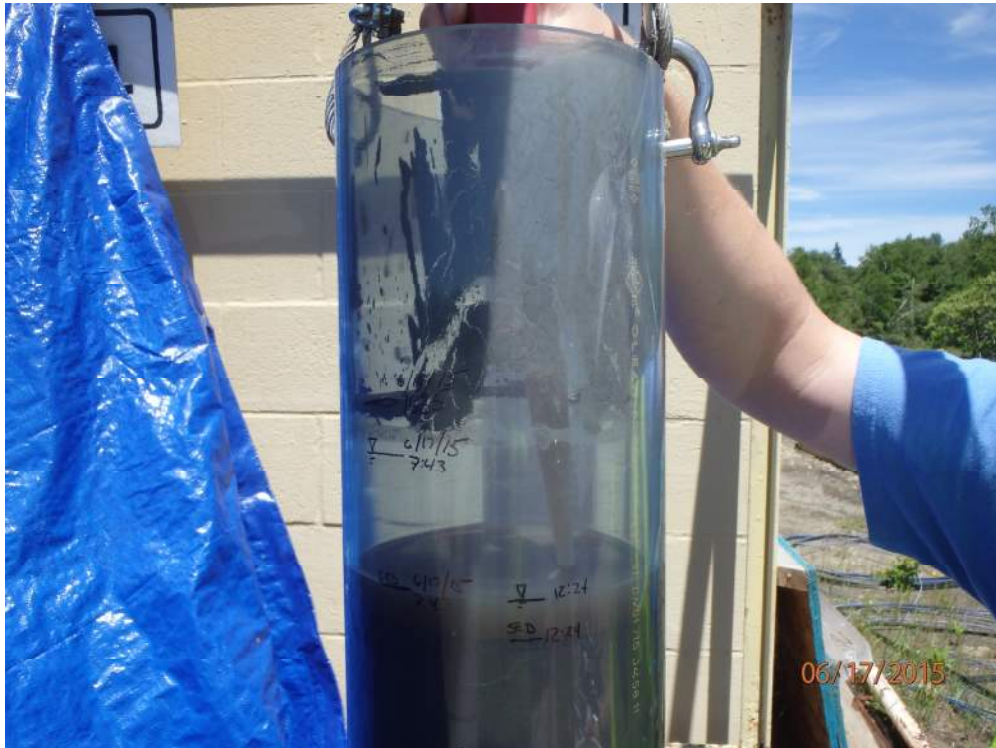
Photo 10: Decanting water from dewatering tube after approximately 21 hours from start of test.
