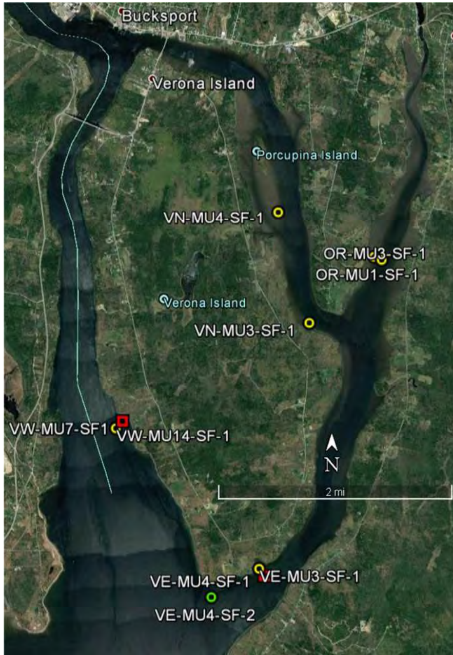
Figure 2-5. Map of coring locations in the area of Verona Island. Yellow dots indicate push cores, green dots indicate gravity cores, and red squares indicate unsuccessful core locations.
