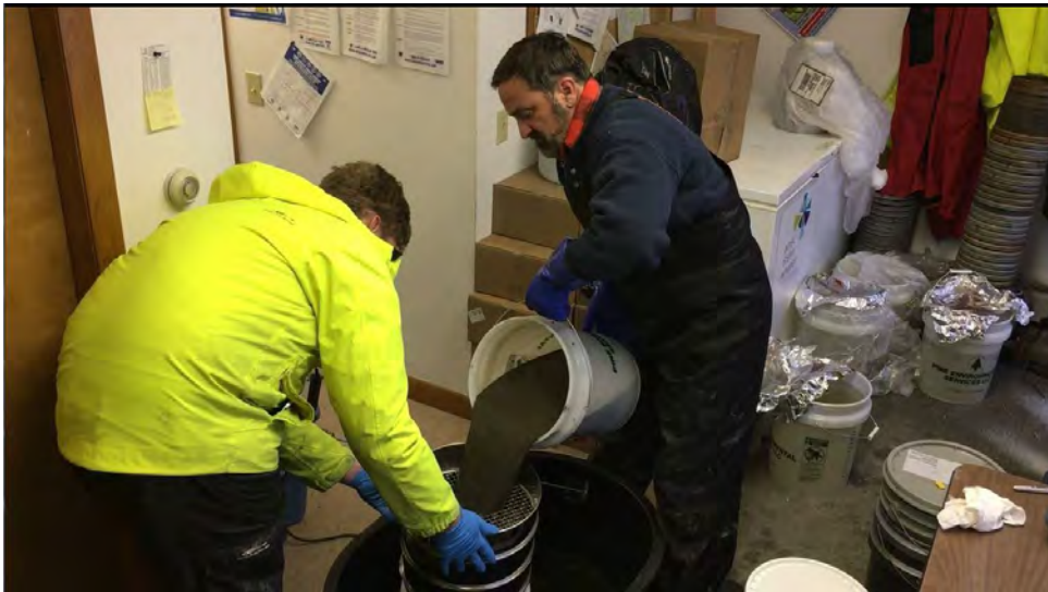
PHOTO 6: Sieve analysis to separate the wood chip and sediment partitions
