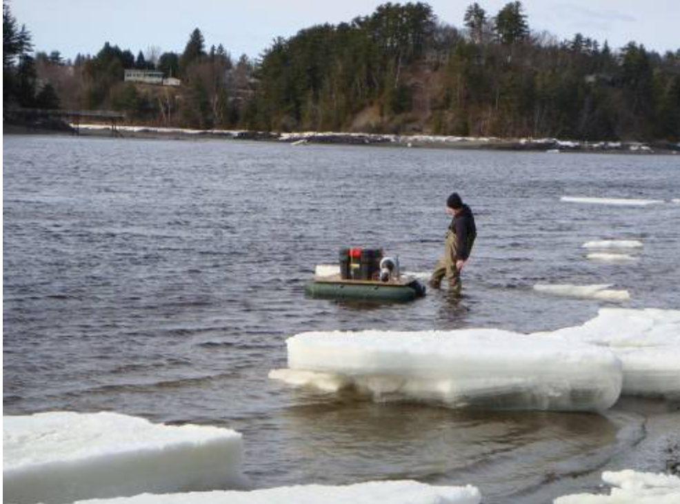
Continuous radon monitoring float – March 2009
