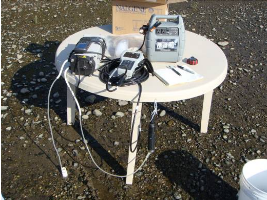
Foreshore porewater collection using well screen
