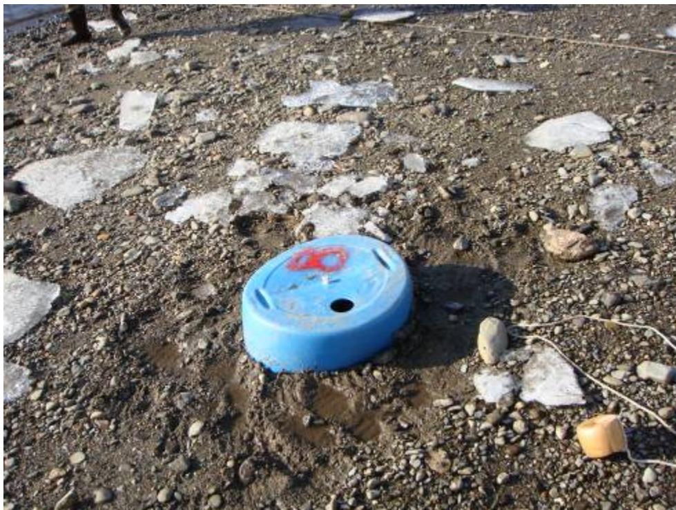
Lee Type seepage meter installed in foreshore prior to rising tide
