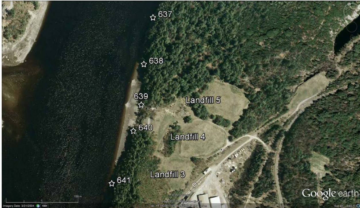
Figure 3-28. Locations of seepage samples collected below Landfills 3, 4 and 5 May 18, 2010
