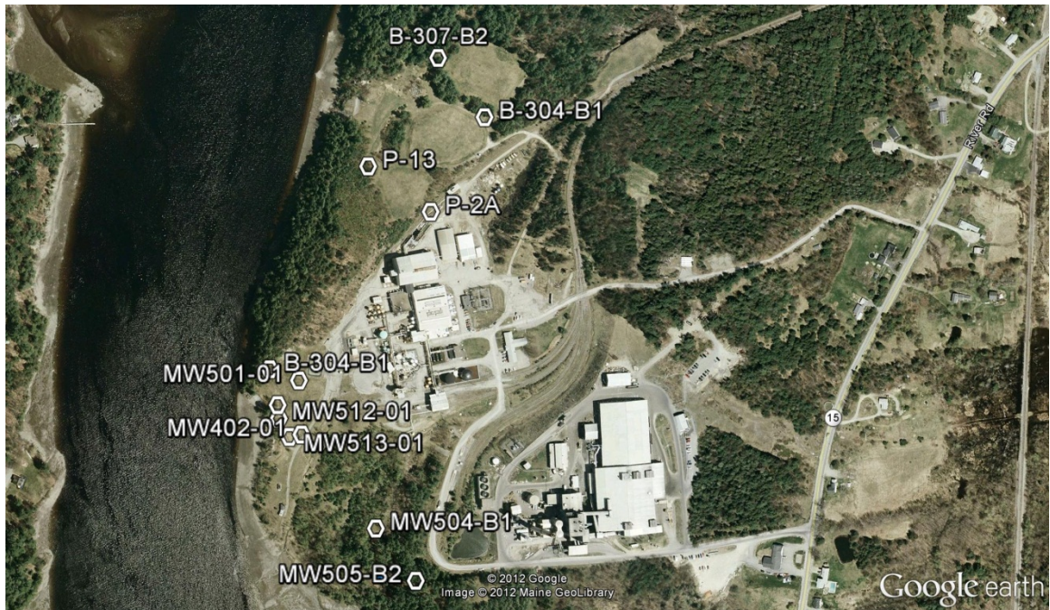
Figure 3-23. Groundwater monitoring wells used to obtain samples for radon analysis, March 2009.
